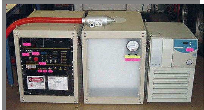
Showing, from left to right, the laser and its controls, the waste management module and the chiller. End-effector (workhead) with its umbilical is resting on top.
