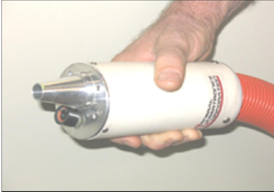
FIGURE 7 Camera-equipped laser tool for confined-space operations.
