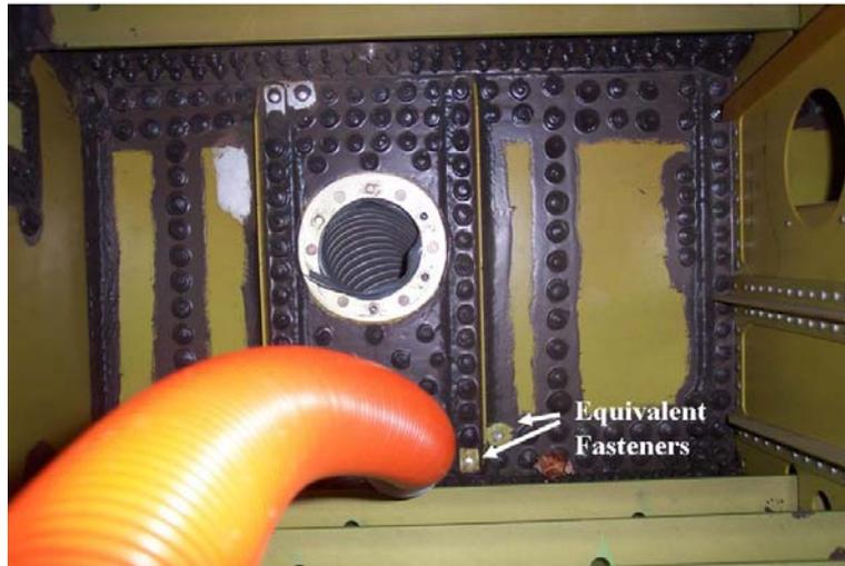
**Figure 8.** Sealant stripped from two fasteners to right of umbilical
