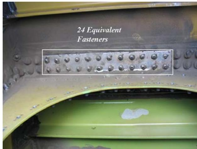
**Figure 9.** Sealant completely removed from a larger area (same area as shown in Figure 2).
