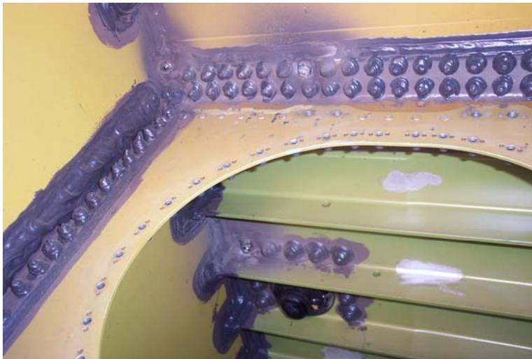
*Figure 2. Sealant covering fasteners in the center wing tank*
