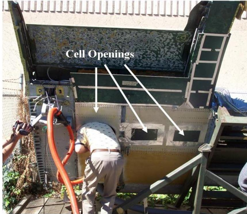
*Figure 4. Port half of the retired center wing tank showing fuel cell openings are barely large enough for an operator*
